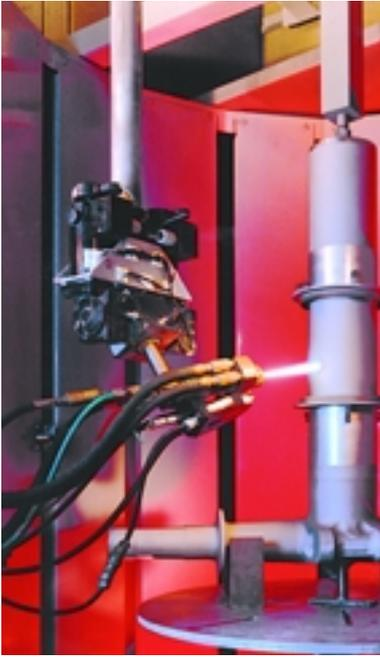
**4** HVOF thermal spray replacement coatings applied on airline landing gear instead of hard chrome plating show better performance.
